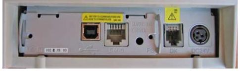
The adapter can replace the existing adapter and is held in place by 2 screws. (Your adapter may not have the network style DM port jack)
